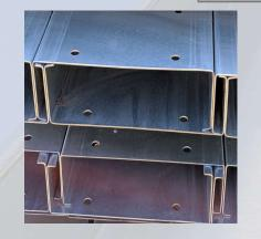
COLD FORMED components are engineered specifically for the building location. The main frame steel will vary from 4" to 24" in depth and 2 ½ to 5" wide, the gauge varies from 16ga to 10ga.
