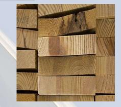
Wood building components are not engineered specifically instead standard codes determine size, species and grade of lumber required. Roof trusses will be engineered.
